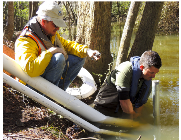
YSI field technicians installing protective casings for a EXO water quality sonde and discrete water sampler suction line.
