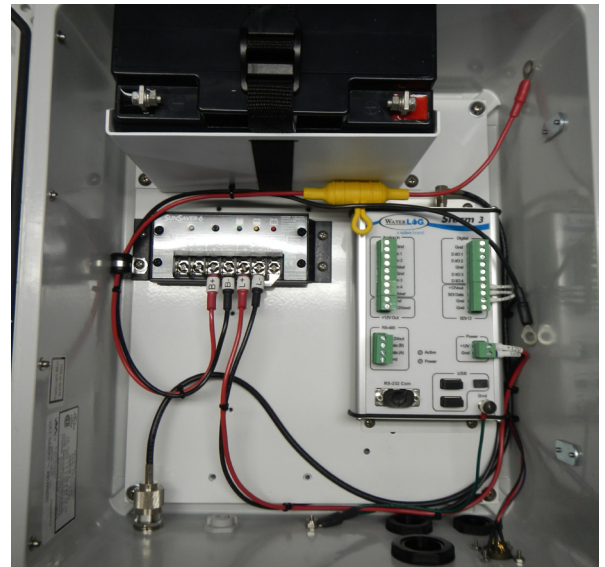
WaterLog Storm 3 Datalogger and control module enabled with water sampler trigger excitation and cellular IP addressable data access for event notification.
